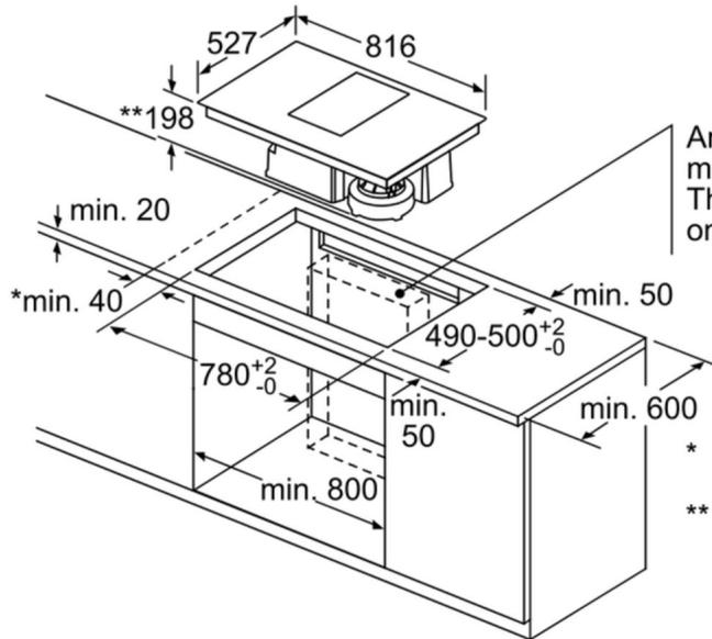
Area for the circulating-air module or the duct.
